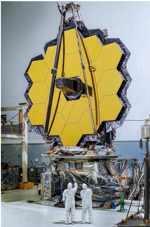
The primary mirror of the James Webb Space Telescope during testing at NASA's Goddard Space Flight Center
