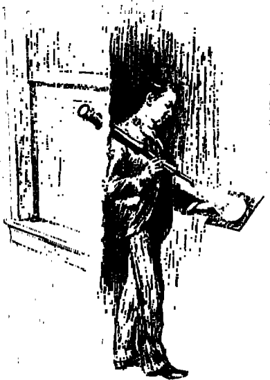
How an image of the sun may be thrown on a screen with a small telescope or a common spy-glass.
