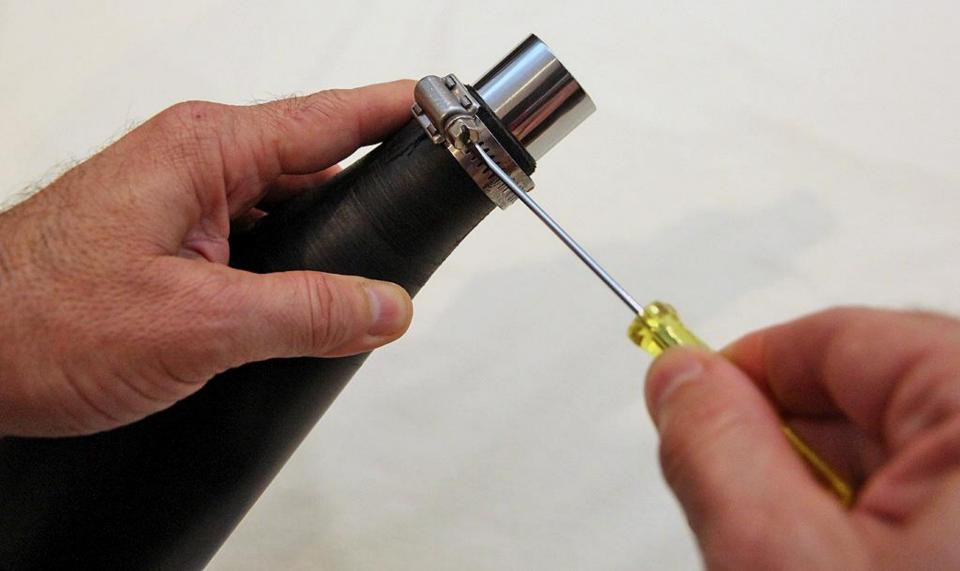
**Step 9.** Turn the funnel wide end up (you might find it easiest to sit in a chair and hold the funnel between your knees). Place the rearprojection screen (or two layers of vinyl shower-curtain liner) over the wide opening; it doesn't matter which side faces down. Lower the large hose clamp over the wide end of the funnel...
