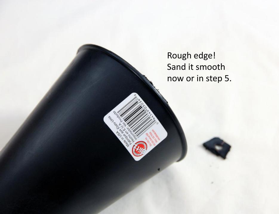
**Step 3.** Using the hacksaw, cut about 7 inches off the narrow end of the funnel so that what's left measures about 10 inches long (use the ruler).
