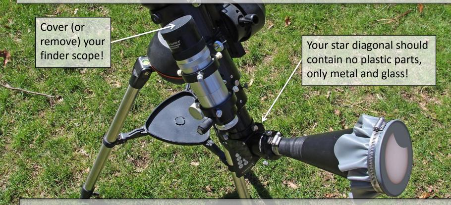
WARNING! ALWAYS SUPERVISE USE OF THE SUN FUNNEL. NEVER POINT AN UNFILTERED TELESCOPE AT THE SUN. SEVERE EYE DAMAGE MAY OCCUR!
