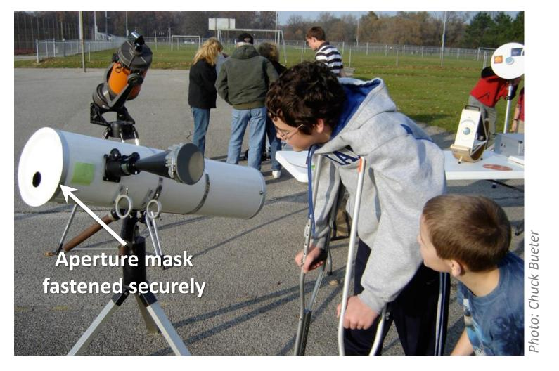
That said, you <u>can</u> use a reflector if you "stop down" the aperture by placing a piece of cardboard over the front end with a small (1- to 2-inch) hole cut off to one side to let in only a little bit of sunlight. Be sure to install the aperture mask <u>before</u> aiming the telescope at the Sun!
